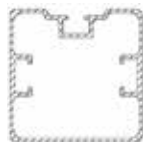
Aluminum posts Reinforced ribbed aluminum profile 80x80 mm
