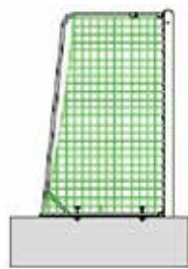
Goal mounted using installation plates / supports
