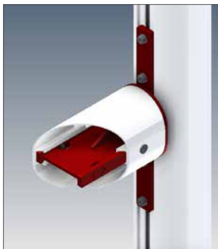
Fixing the crossbar to the post
