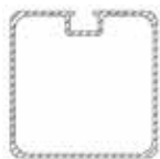
Aluminum posts Standard profile 80x80 mm
